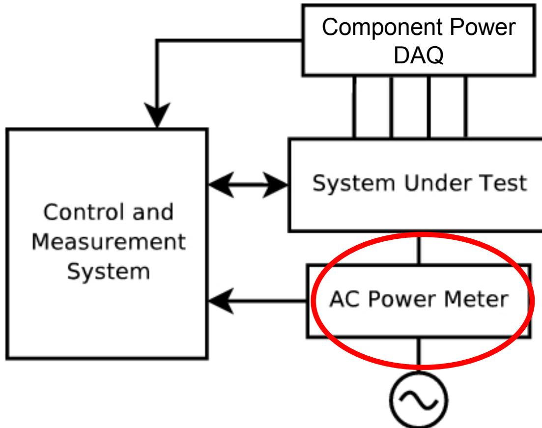
Insert measurement between machine and wall to measure overall power
